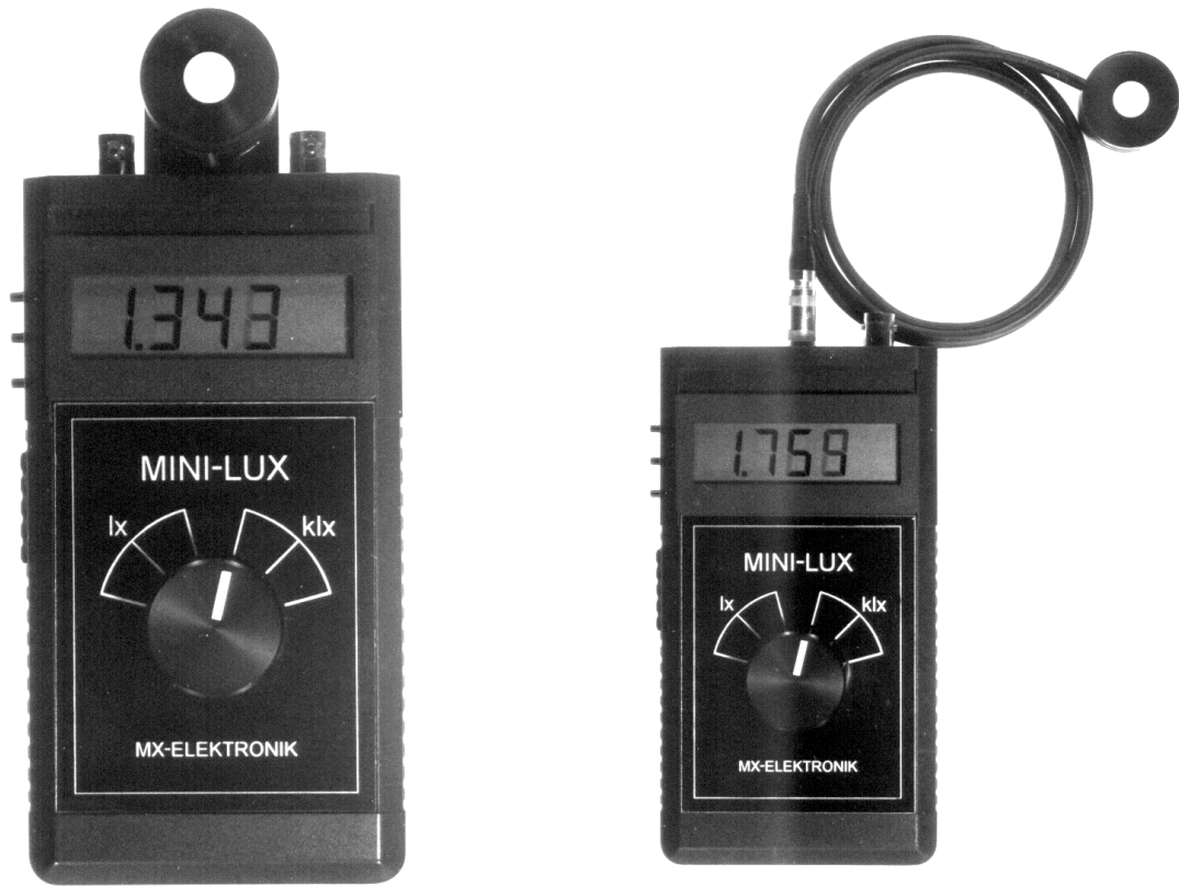
Fig. 1. The MINILUX- device with photosensor (silicon-cell with V(\lambda) - and cosine-correction in accordance to DIN 5032, class B)
