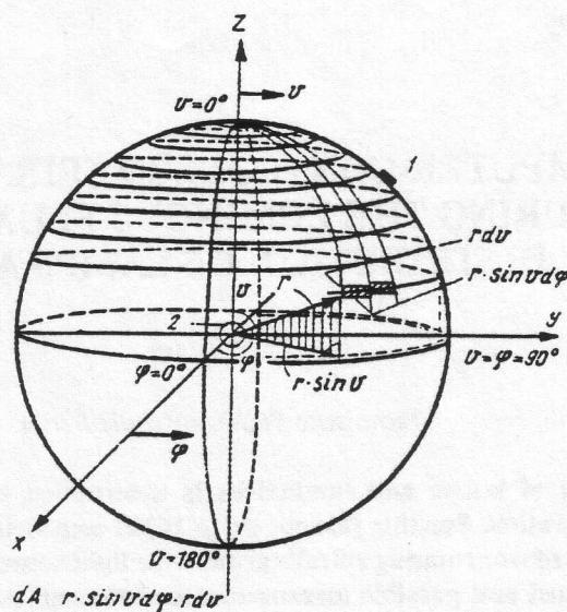
Fig. 1. Principle of spiral scanning: 1) photodetector; 2) light source.
