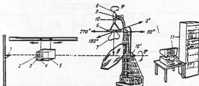
Fig. 3. Design diagram of a photometer with a rotary mirror:
