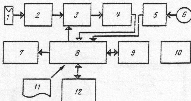
Fig. 5. Microcomputer-controlled electronic integration of luminous flux. 1) Sensor; 2) Input amplifier; 3) Sample and Hold circuit; 4) Analog/Digital Converter; 5) I/O; 6) Positioning indicator; 7) Printer; 8) Microcomputer; 9) Rapid arithmetic processor; 10) Power supply; 11) Programme; 12) Monitor with keyboard.
